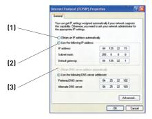
5. If "Use the following IP address" (2) is selected, your Router will need to be set up for a static IP connection type. Write the address information the table below. You will need to enter this information into the Router.
